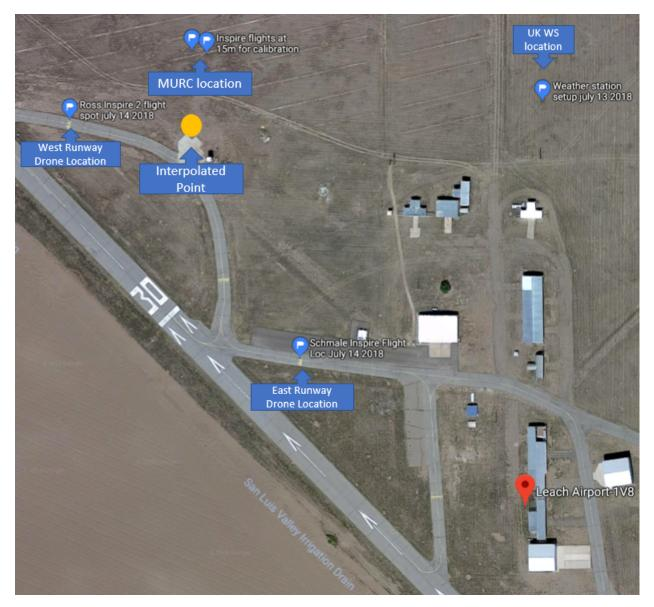
Figure 4.6: Satellite image of the sampling region with sensor locations marked with blue pins. A potential interpolated point is marked in yellow.
