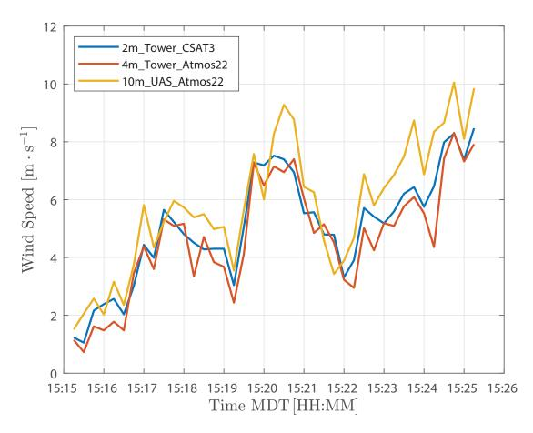
Figure 4.7: Comparison of wind speed measurements on the flux tower for a height of 2 m (CSAT3 sonic anemometer, yellow), 4 m (Atmos22 sonic anemometer), and 10 m (UAS with Atmos 22 sonic anemometer.
