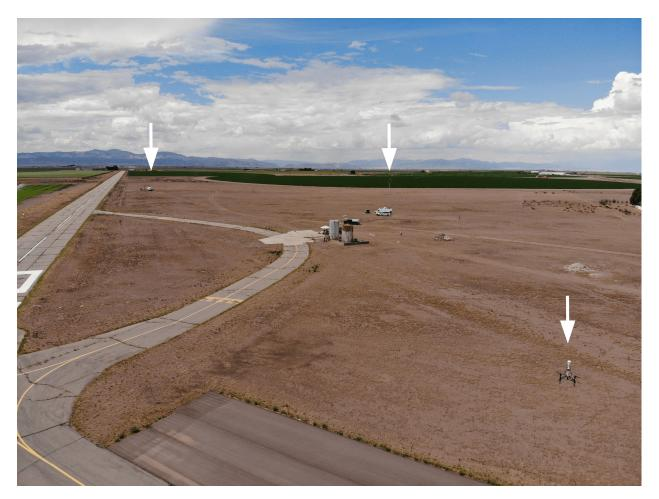
Figure 4.4: Simultaneous flights with sensors in a triangle formation (white arrows). Both UASs were operating off of marks on the taxiway, and the MURC tower was stationed north of the UAS operations.
